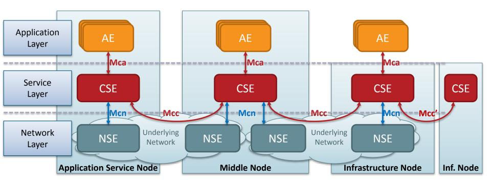
Multiple protocol bindings (HTTP, CoAP, MQTT, or WebSocket) over Mca, Mcc, Mcc'
